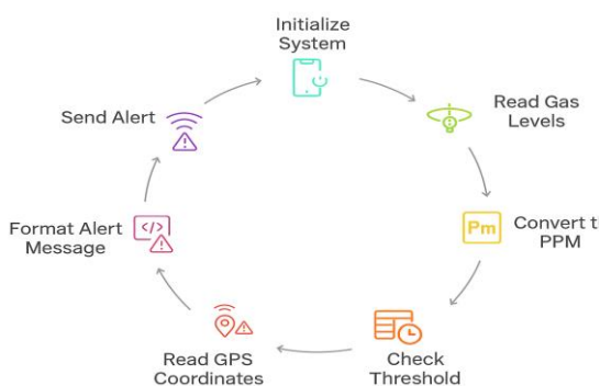
Dual-Sensor LPG & NPG Leakage Detection Cycle
