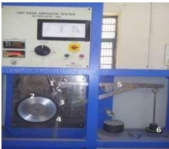
Figure.2: Rubbing wear testing equipment using dry sand and rubber wheels
