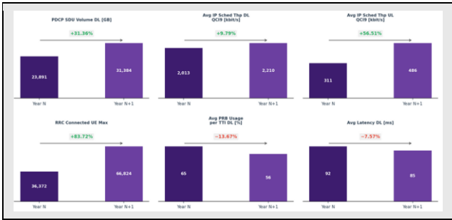
Fig. 2. Six-panel year-on-year KPI comparison bar charts for 4G LTE: (a) PDCP DL Volume, (b) Avg DL Throughput QCI9, (c) Avg UL Throughput QCI9, (d) RRC Connected UE Max, (e) Avg PRB Usage DL, (f) Avg DL Latency. Year N shown left; Year N+1 shown right with delta annotation.
