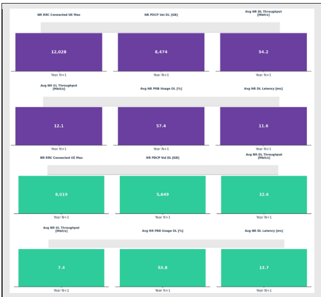
Fig. 3. Six-panel year-on-year KPI comparison bar charts for 5G NR n78 (upper row) and n40 (lower row): NR RRC UE Max, NR DL Data Volume, NR DL Throughput, NR UL Throughput, NR PRB Usage DL, NR DL Latency.
