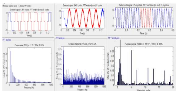
Figure 8: Comparison of filter performance
