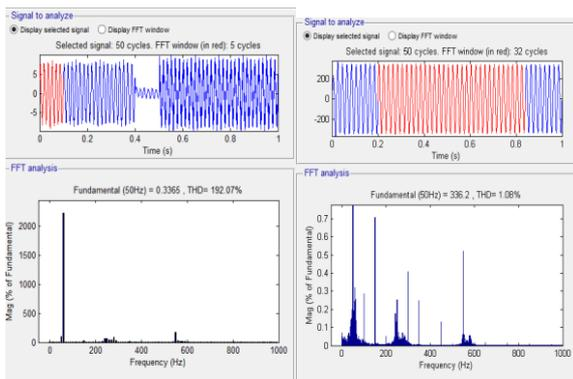
Figure 13: Voltage Harmonics before and after filtering
