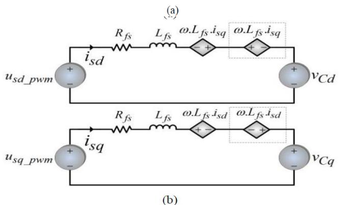
Fig. 2. Series converter: (a) Signal flow graph of the current controllers and average model; (b) Model of the uncoupled system in SRF dq-axes.
