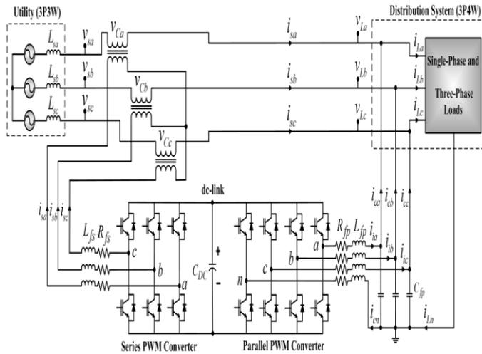
Fig. 1. 3P4W distribution system based on UPQC topology Connected to 3P3W power system.
