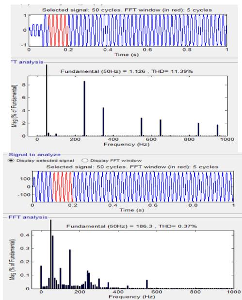
Figure 14: Current harmonics before and After filtering
