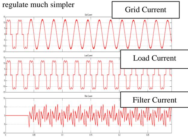
Figure 7: compensation in the volterra filter
