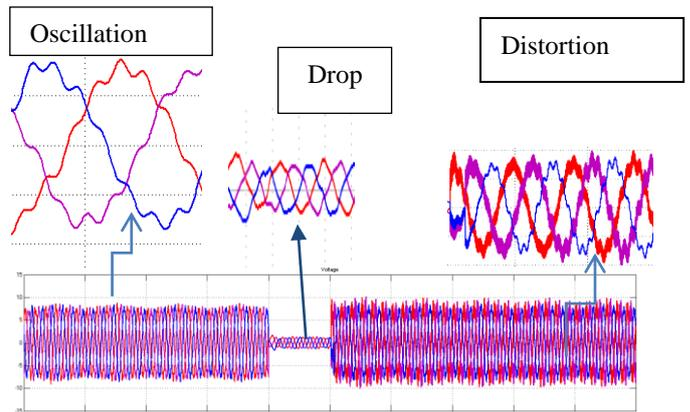
Figure10: Problems in transmission line due to load unbalance
