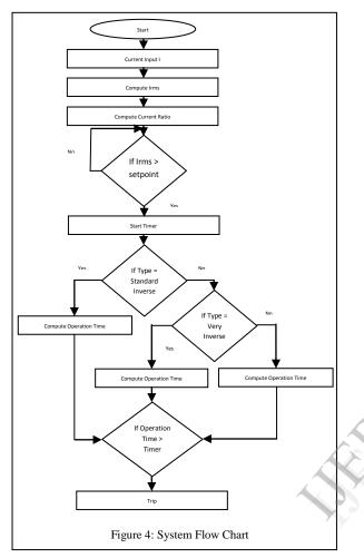
Implementation of IDMT characteristics can be carried out by computing the Root Mean Square i.e. RMS value of the input current. The RMS value is then compared with setpoint value and then based on the timer value, characteristic is identified and relay trip logic is activated. Relay characteristic is identified based on comparison of operation time and timer value. The whole process can be represented in the form of a flowchart as given in Figure 4 [7], [8].
