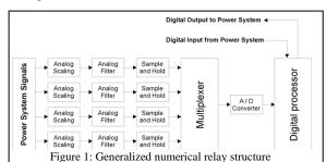
1. *Isolation and analog signal scaling:* Current and voltage waveforms from instrument transformers are acquired and scaled down to convenient voltage levels for use in the numerical relays.
