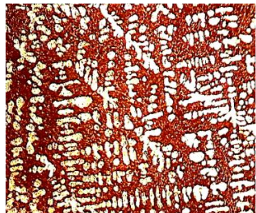
200X as etched Fig.3 Al -Si – 4% \text{TiB}_2 .
