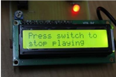
Figure 8. LCD Display Indicating that the Text has been converted into Speech
