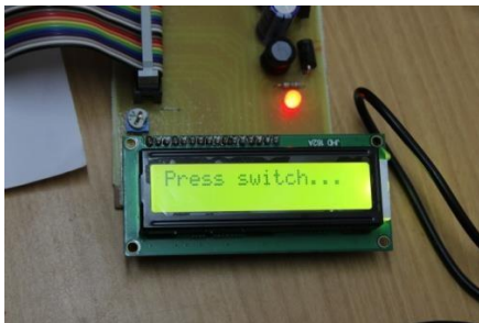
Figure 5. LCD Display Indicating to Press a Switch
