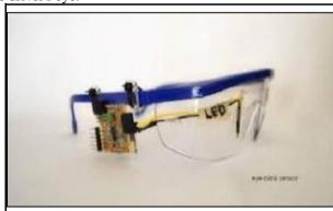
Fig. 1 Drowsiness Detection System assembled on spectacles
