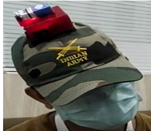
Fig. 12: When head tilted towards left, device gives alert.
