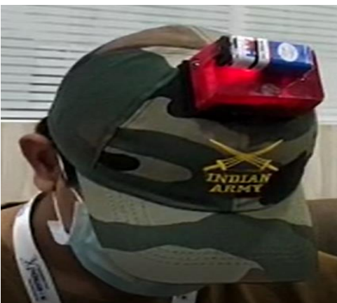
Fig. 11: When head tilted towards downward, device gives alert.
