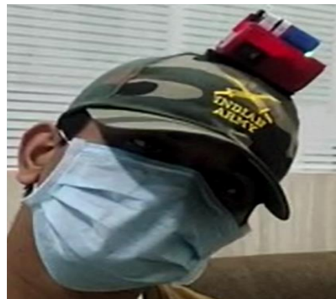
Fig. 13: When head tilted towards right, device gives alert.
