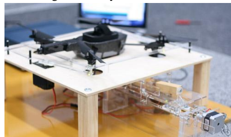
Fig1: Endless Flyer: automatic battery replacement platform enables UAV to fly continuously without requiring manual battery replacement.
