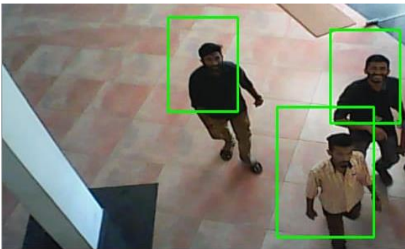
Fig 2: Human Detection using Haar Cascade Algorithm
