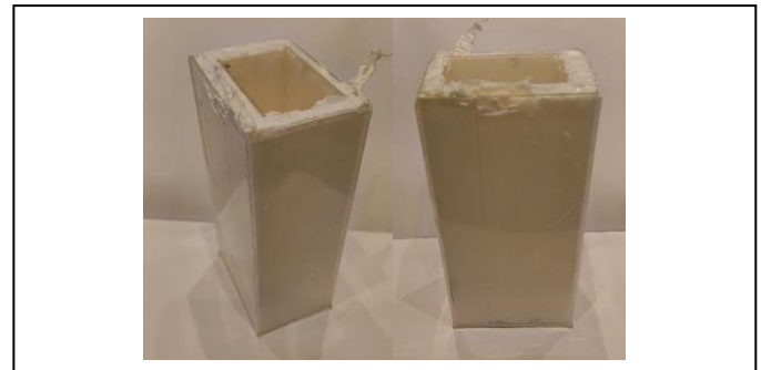
Fig. 7. PU Foam insulation within acrylic sheets
