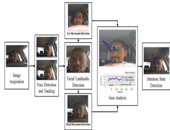
Fig 6. Schematic diagram of driver's attention monitoring system
