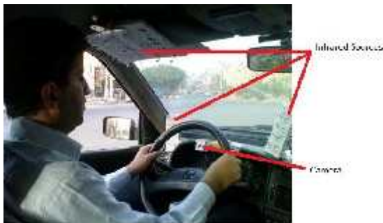
Figure 2. The hardware of the implemented system.
