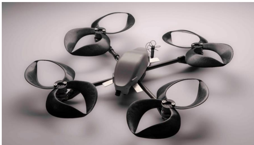
Figure 2. A toroidal (double-helix) propeller. Note the absence of free blade tips — each blade loops into the other (image: MIT Lincoln Laboratory).
