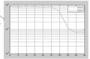
The above graph depicts graph of Frame Error Rate [FER] versus Output Signal-to-Noise ratio [SNR] for 1\*1\*1 and 1\*2\*1 transmitter and receiver antenna inputs with the use of ordered subcarrier pairing technique for Rician noise channel model.
