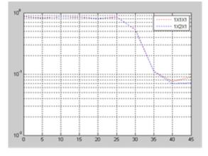
The above graph depicts graph of Frame Error Rate [FER] versus Output Signal-to-Noise ratio
