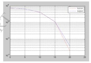
The above graph depicts graph of Frame Error Rate [FER] versus Output Signal-to-Noise [SNR] ratio for 1\*1\*1 and 1\*2\*1 transmitter and receiver antenna inputs with the use of ordered subcarrier pairing technique for AWGN noise channel model.
