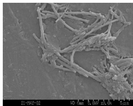
Fig. 3. Lengths of nanotubes after grinding
