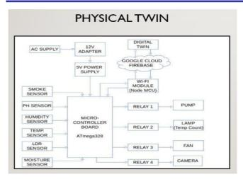
In case of the digital twin the data which is stored in the cloud are displayed with the help of the software. Also we can control the various actions like pumping, faning..etc with the help of this software. Using this android application any person can monitor this physical twin from anywhere.
