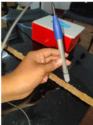
Fig.3 (a): Ag/AgCl reference electrode Fig.3 (b): Working electrode Fig.3 (c): Test set-up Fig.3 (d): Mobile app
