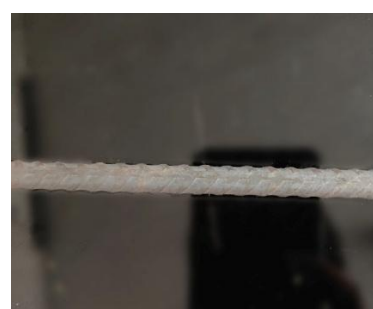
Fig.2 (b): Non corroded 10 mm \phi bar
