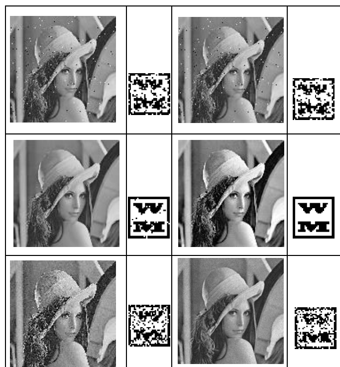
Fig. 4. Watermark Attack analysis ( Salt & Pepper, Histogram equalization, Wiener filtering, Contrast adjustment, Image sharpening, Poisson attack)
