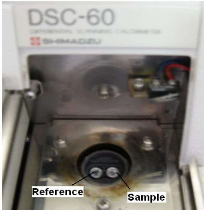
Fig.2: Reference and sample aluminum pans in DSC
