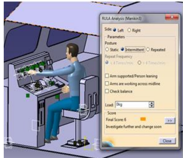
Fig. 13 RULA result of the existing assembly
