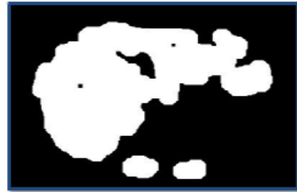
Fig. 6. Resulted Image of applying Opening function to separate the regions of different organs.
