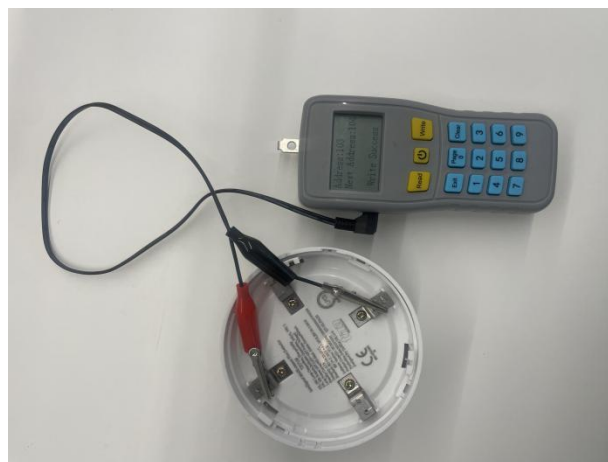
Figure 3. Handheld programmer being used to read and modify device addresses on-site.
