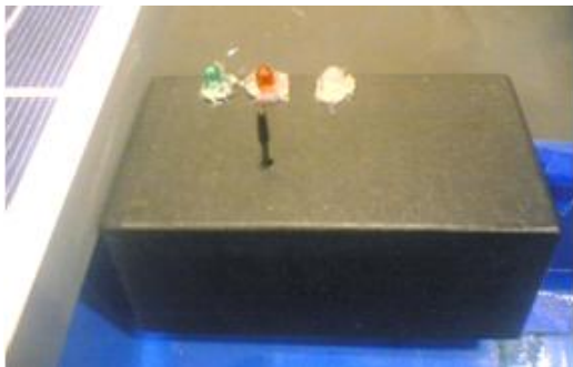
Figure 4: Sealed box with LED's used as an indicator
