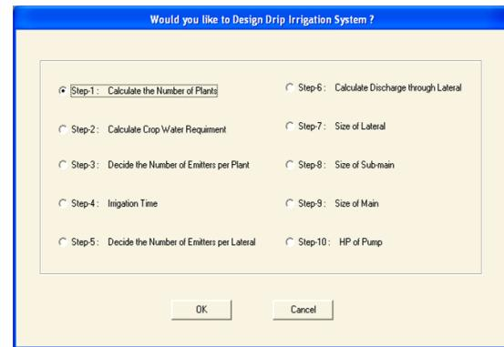
Fig. 2: Steps involved in design of drip irrigation system
