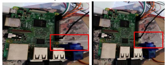
Fig 11: Servo Motor with 0° and 90° rotation
