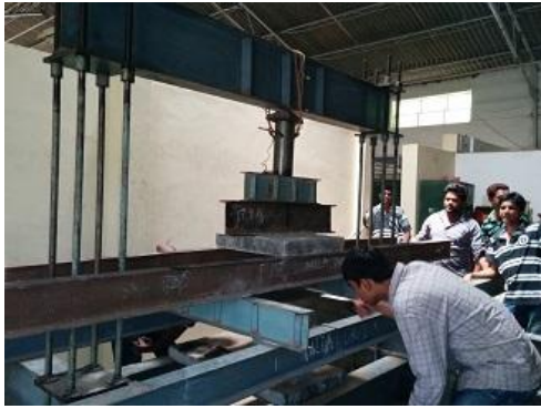
Figure 3- Flexural strength test of Slab specimen
