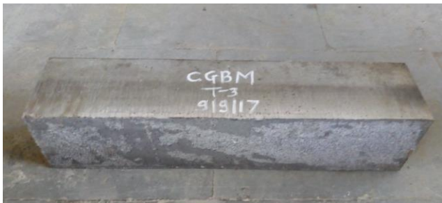
Fig. 6. Flexural beam specimen
