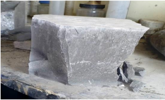
Fig. 4. Cube failure pattern.
