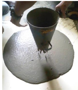
Fig. 1. Flow table test.
