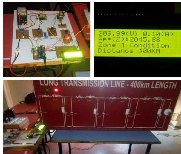
Fig. 8.2 when fault is applied on transmission line at 100Km.
