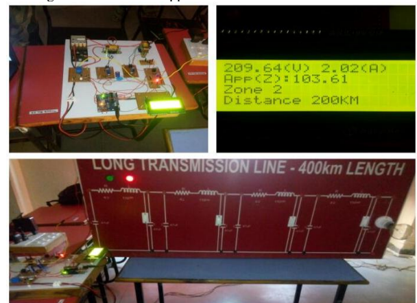
Fig. 8.2 when fault is applied on transmission line at 100Km.
