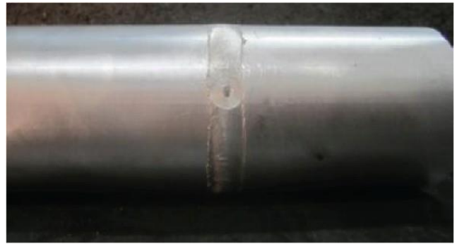
Slight weld flash on trailing edge that has exhibited more good quality weld at 1400 rpm speed
