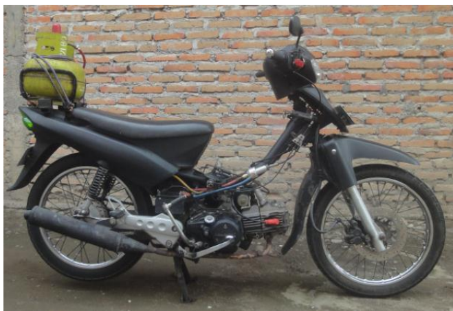
Figure 3. LPG fuelled 112 cc single cylinder four stroke motorcycle
