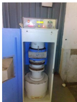
Fig. 3 Test specimen under compression test
