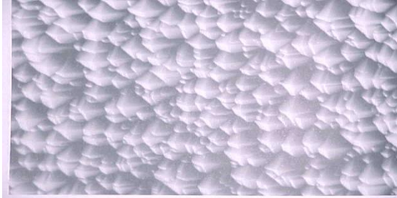
Fig 1: SEM photograph of pyramidal structure formed on the silicon wafers
