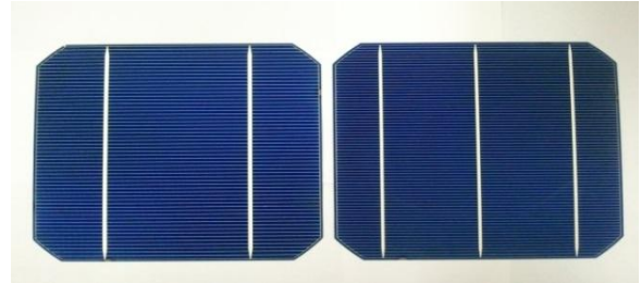
Fig 3.a: Front side pattern comparison – 2 Busbar vs 3 Busbar
