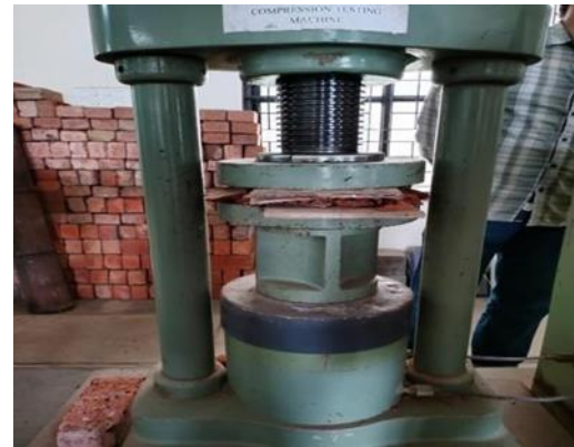
Fig 4.2 Compressive strength testing of brick
