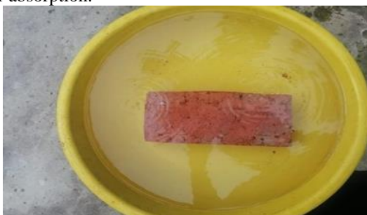
Fig 3.1 Brick immersed in water for absorption test
