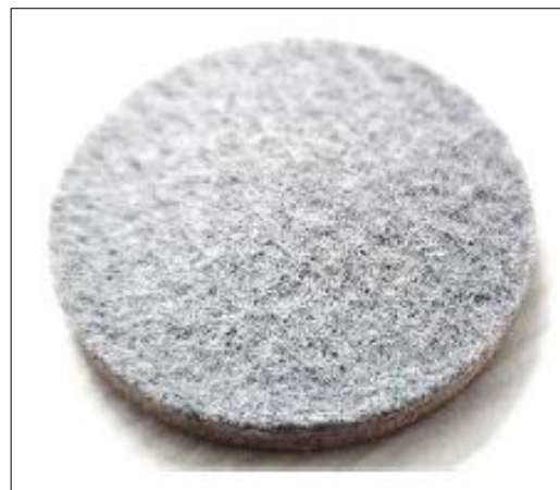
Figure 8: Sample for Sound Absorption Coefficient (SAC)
