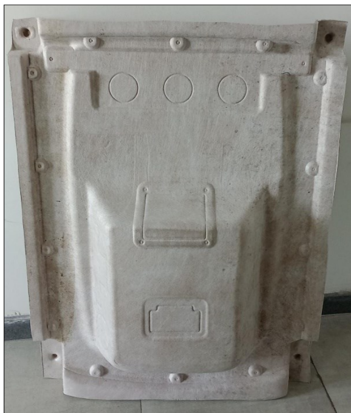
Figure 7 (b): Developed Roof Liner made up of 50% Jute and 50% Polypropylene (PP) for M/s Sonalika Tractor
