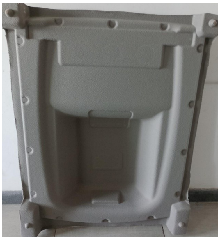
Figure 7 (a): Front side of moulded roof liner
