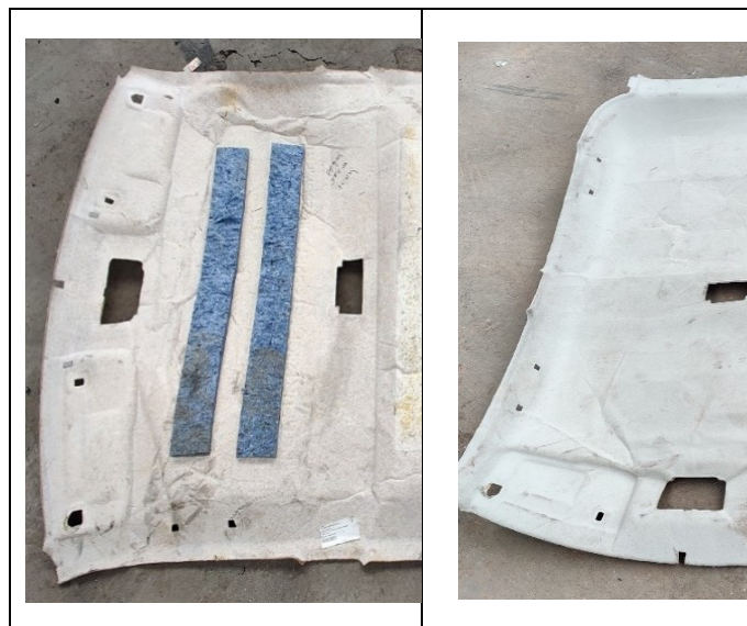
Figure 1: Collected roof liner samples from used cars
