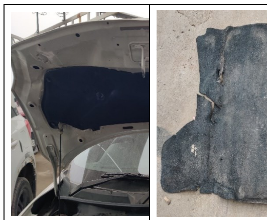
Figure 2: Collected engine shield samples from used cars
