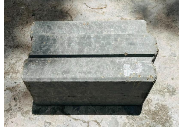
Fig 7: Images of Interlocking Brick after Efflorescence Test
