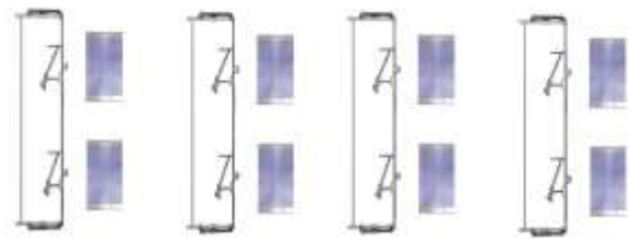
Fig. 15. Solar roof collectors when using four heliostats
