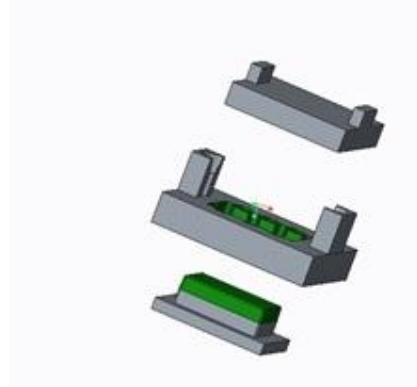
Fig.13. Exploded view of Die assembly
