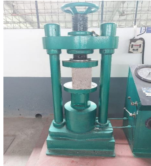
Figure 3: Casting ,curing and strength testing of specimens
