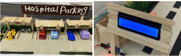
Fig 12. LCD display shows slot 2 is available and also LED is off
