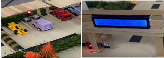
Fig.11 LCD display shows Slot 2 is occupied and LED glows.
