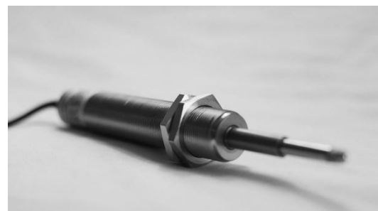
Fig 5.3 Linear Variable Differential Transformer
