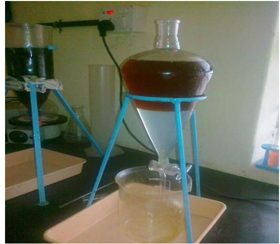
Fig. 6: Washing with hot water
