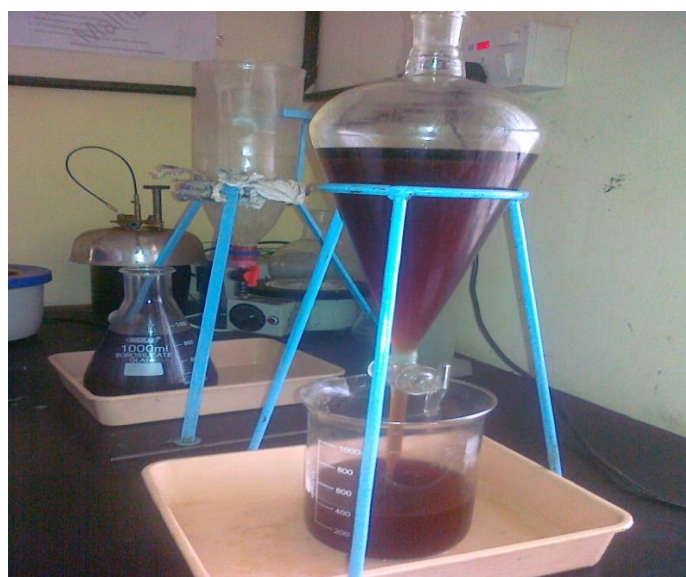
Fig. 4: Separation of free fatty acid
