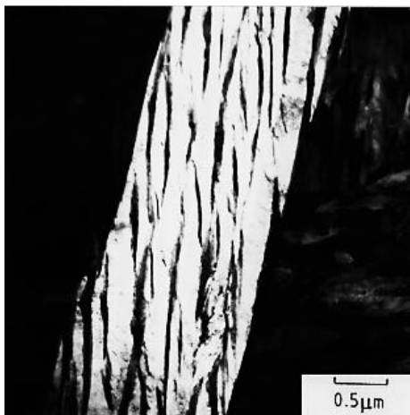
Figure 4.1: Transmission electron micrograph of a sheaf of Carbide-free upper bainite, consisting of fine ferrite platelets separated by films of carbon-enriched retained austenite [7, 11, 15].
