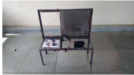
Fig.2 : Completed automatic rain sensing window
