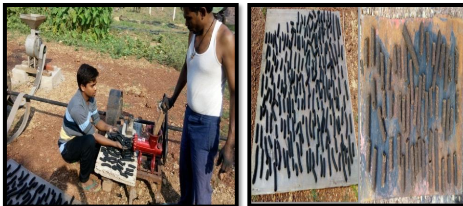
Fig.2: briquette production through rotary unit
