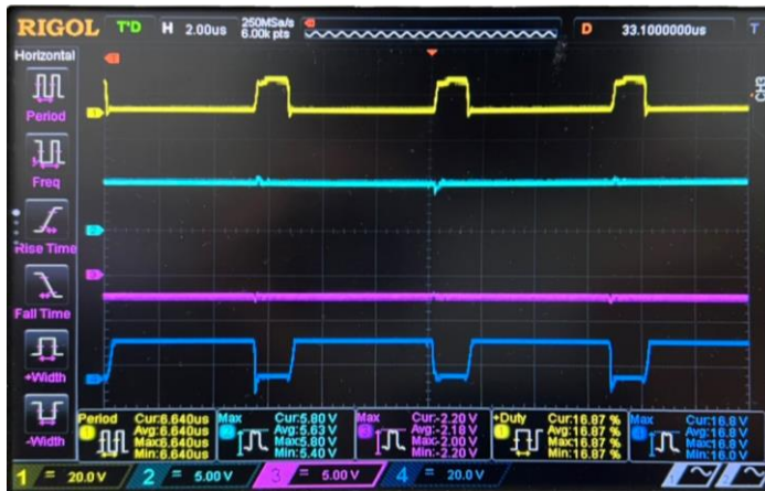
Fig. 13. The test results of the integrated circuit working in buck mode of the Cuk mode.
