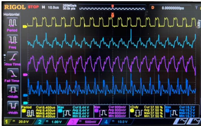
Fig. 9. The test results of the integrated circuit working in buck mode.
