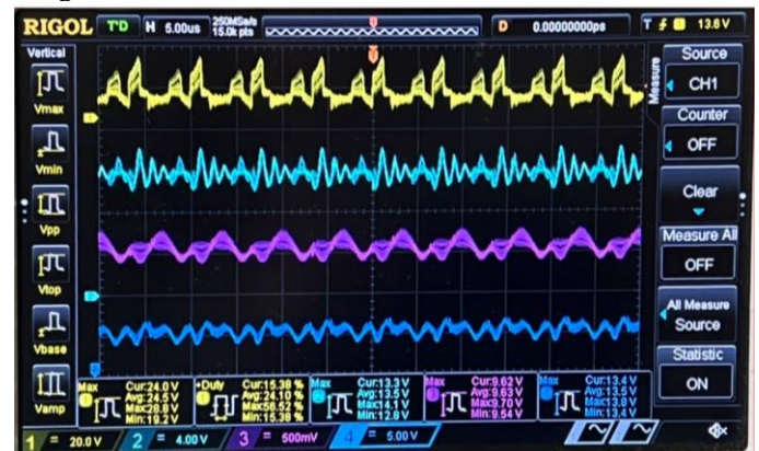
Fig. 11. The test results of the integrated circuit working in buck mode of the buck/boost mode.
