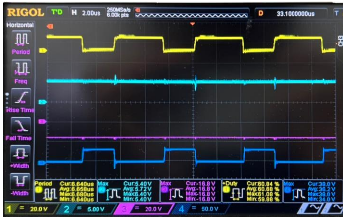
Fig. 14. The test results of the integrated circuit working in boost mode of the Cuk mode.
