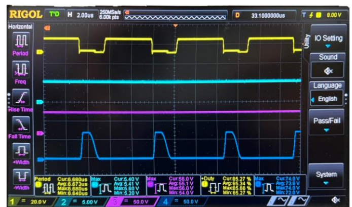
Fig. 12. The test results of the integrated circuit working in boost mode of the buck/boost mode.
