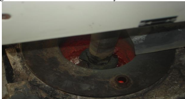
Figure 1: Mixing of SiC in Al alloy
