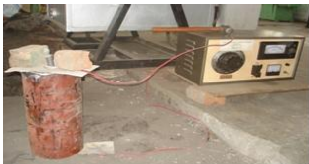
Figure 3: Experimental set up for electric current passing through sand cast
