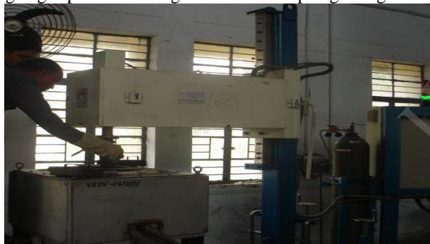
Figure 2: Experimental set up for stir casting
