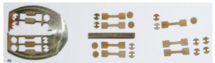
Fig 7 Scheme for extraction of miniature test specimen (7a) Pictorial representation of boat sample from HAZ region & kerf width and 3mm disk specimen, miniature size tensile specimens, 3mm hour glass shaped fatigue specimen and miniature charpy impact test specimen. (7b) preparation of miniature test specimens by EDM
