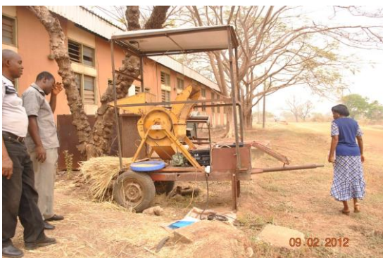
Figure 1: picture of the photovoltaic powered tractor-drawn rice threshing machine
